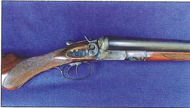
Photo 1: This 10 gauge F Grade, SN 89971, was manufactured in 1901 and restored in 2020. The stock is figured English walnut with a Prince of Wales grip and 22-point checkering. The 32-inch barrels are made of very fine Damascus steel. Both barrels are choked extra-full. log excerpt describes the new F Grade.
